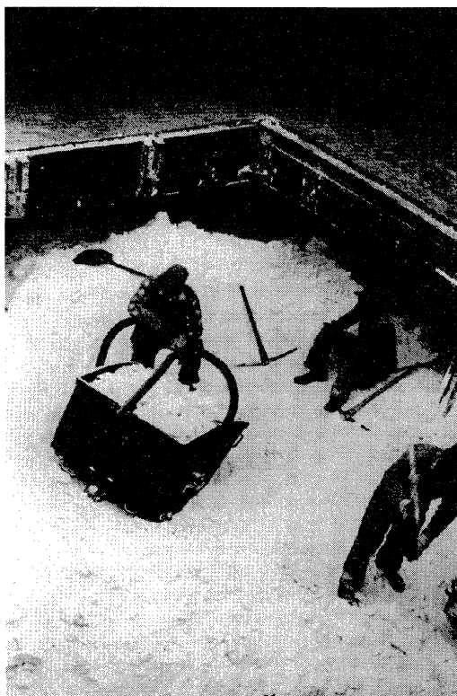
Figure 6.50. Manually unloading a shipload of caked sylvite.
