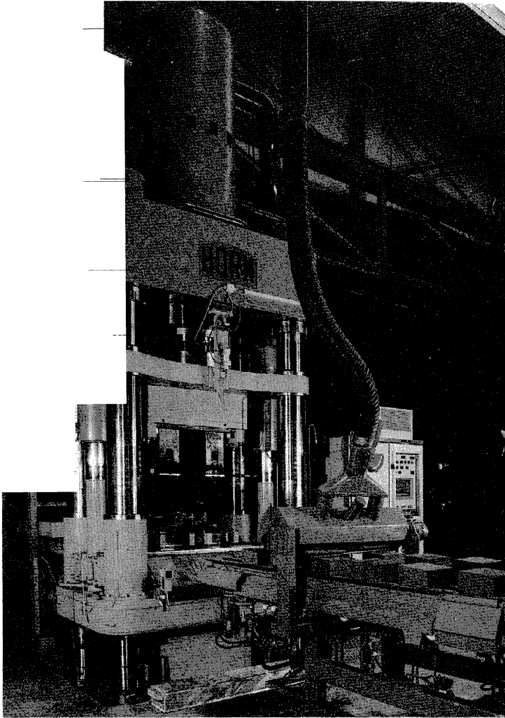
Typical vertical hydraulic press for the manufacture of refractory brick (Horn, Worms, Germany).
